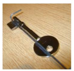
Insert the long reader wire into the hole in the wire handle and gently feel under the rear of each lever and read off the angle on your chart.
